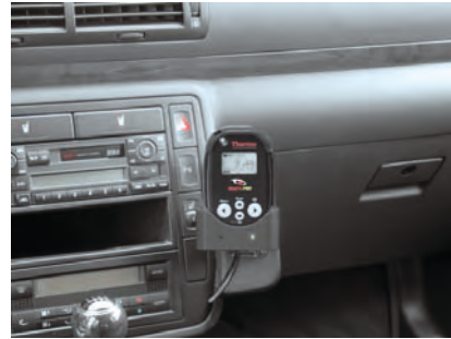
RadEye car adapter for mobile area survey applications
